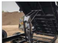
SCISSOR LIFT WITH POWERFUL CYLINDER
