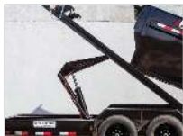
SCISSOR LIFT WITH POWERFUL CYLINDER
